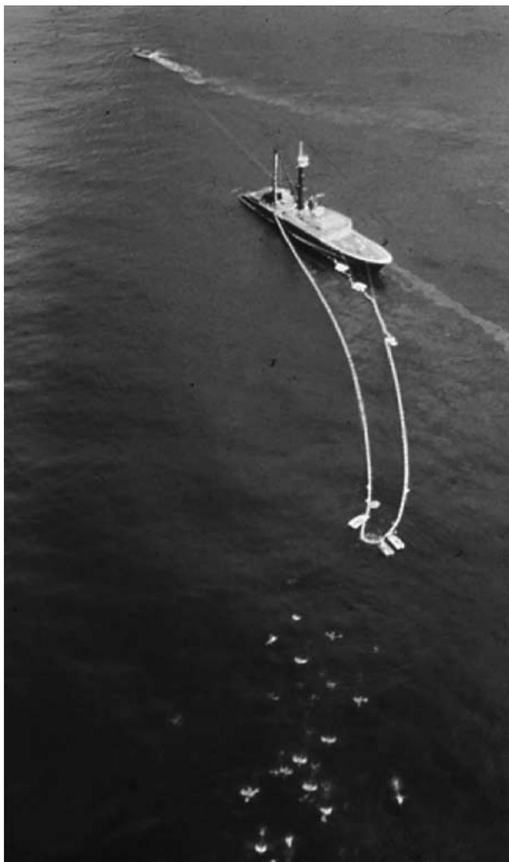
**Figure 4** The 'backdown' manoeuvre used in tuna purse-seining.
