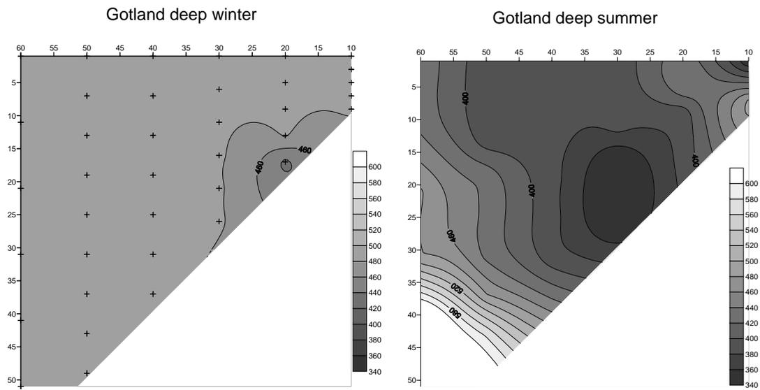
Figure 5. Range in m of a pinger 2 m above the bottom in the Gotland deep in the Baltic. For interpretation of the map see text.
