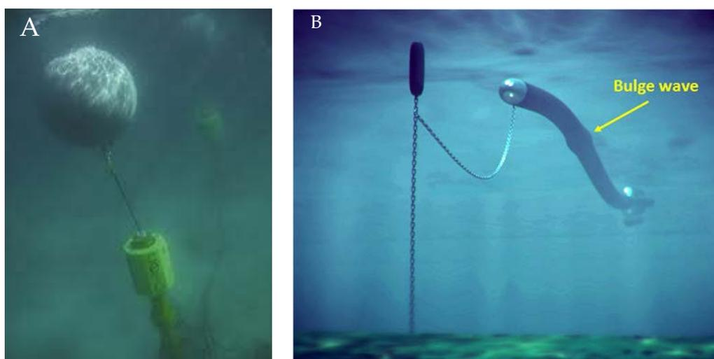
Figure 5.6. Examples of A) a submerged pressure device: © CWE 2011. A CETO™ device. B) an example of a completely different device design: © Checkmate Sea Energy 2012. Artist's impression of an Anaconda™ device.
