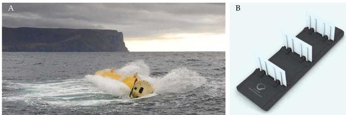
Figure 5.3. Examples of surface attenuators: A) © APL 2012. An Oyster device protruding from the water at the EMEC test site, Orkney, UK; B) © AW Energy 2012. A 3x 100KW WaveRoller prototype.
