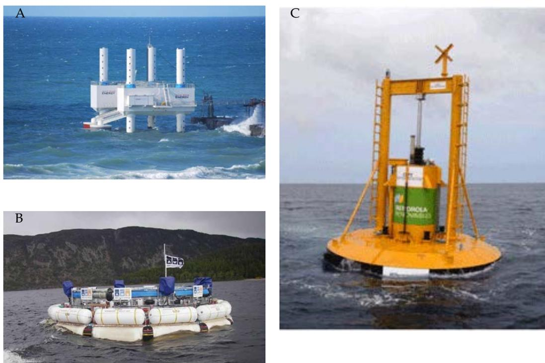
Figure 5.2. Examples of point absorbers: A) © Wave Star A/S 2011. The Wave Star™ 1:2 scale demonstration plant in Hanstholm, DK; B) © AWS Ocean Energy 2010. A 1:9 scale model of the AWS-III™ device being tested in Loch Ness, Scotland, UK; C) © OPT 2012. A PowerBuoy™ device.
