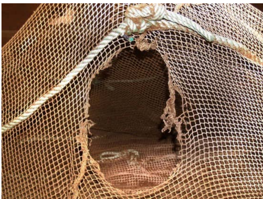
Figure 9.2. Typical predator hole in a net (photo credit: Knox Nets; taken from Northridge et al. , 2013).
