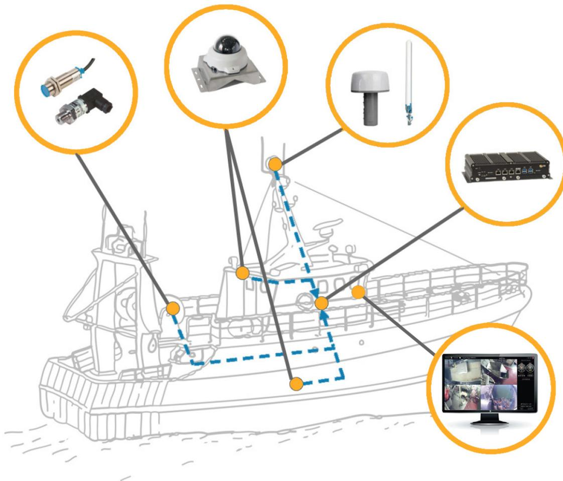
Figure 5. A diagram of a fishing vessel installed with a full electronic monitoring system (courtesy of Anchorlab, 2019).
