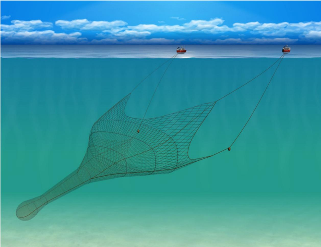
Figure 8. Illustration of a midwater pair trawling team in operation (Source: [www.Cornwallgoodseafoodguide.org](http://www.Cornwallgoodseafoodguide.org), accessed 5th March 2020).
