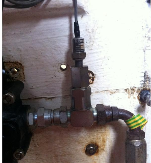
Figure 4. A hydraulic pressure sensor installed on a fishing vessel, to detect hauling activities.
