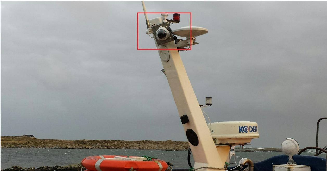
Figure 2. CCTV cameras installed on a small inshore commercial fishing vessel.
