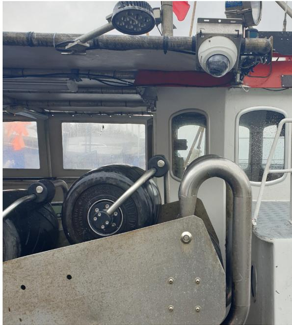
Figure 9. A Danish gill netting vessel fitted with Electronic Monitoring equipment (courtesy of Lotte Kindt-Larsen, 18th February 2020)
