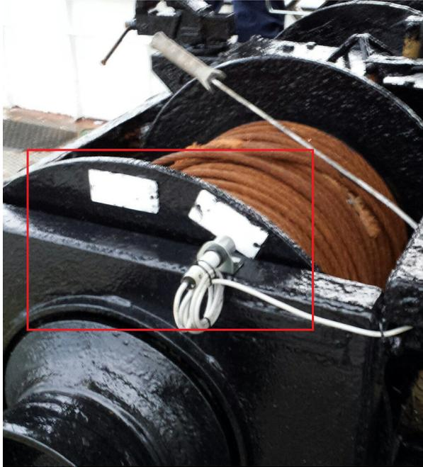
Figure 3. A winch rotation sensor for detecting fishing activities, installed on an inshore trawler.
