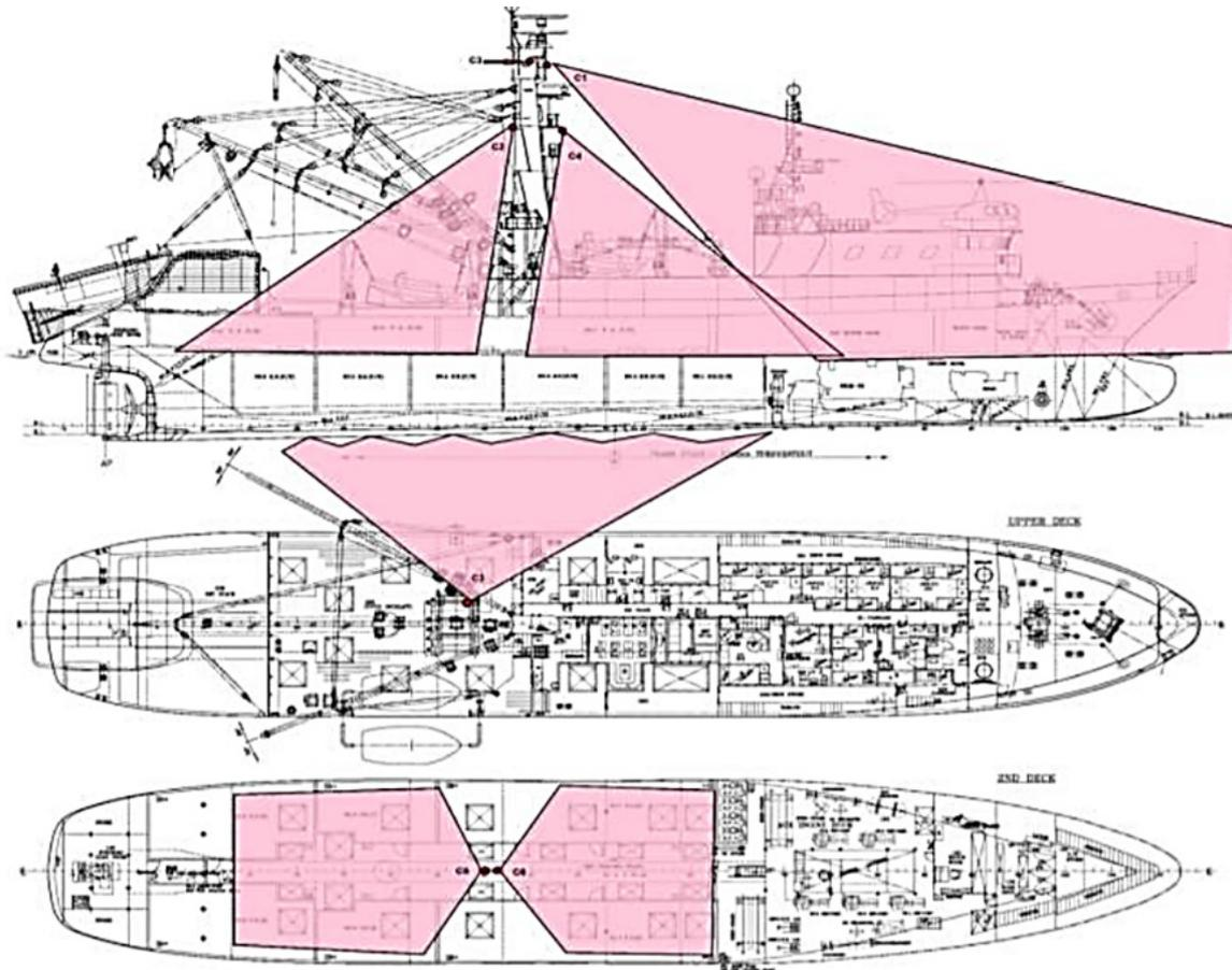
Figure 6. A vessel installation plan for a large offshore tuna purse seine vessel. The pink shaded areas show the field of view for each installed CCTV camera and how they cover the main activity areas associated with the fishing activities and catch processing (MRAG, 2017).
