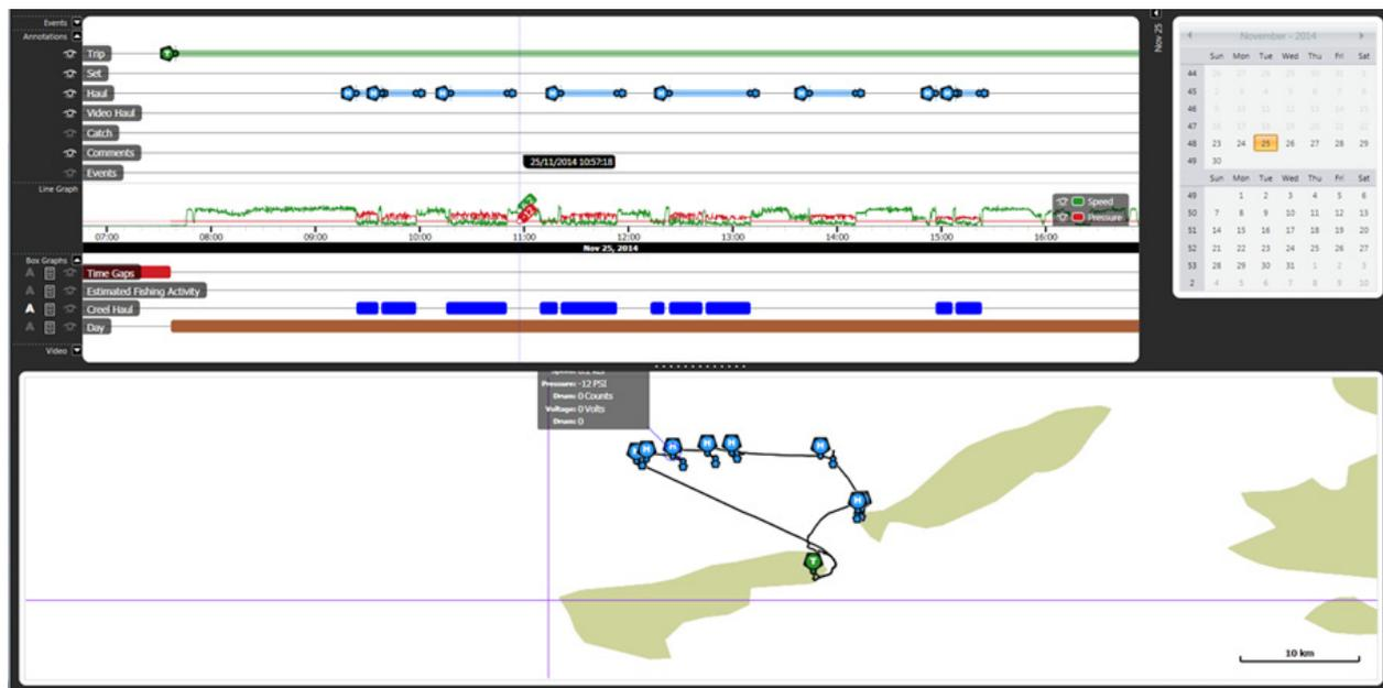
Figure 7. The track of a shellfish creel fishing vessel for a single fishing trip. The speed and hydraulic sensor readings are displayed on the line graph and are used to identify gear hauling positions (Course *et al.*, 2015).
