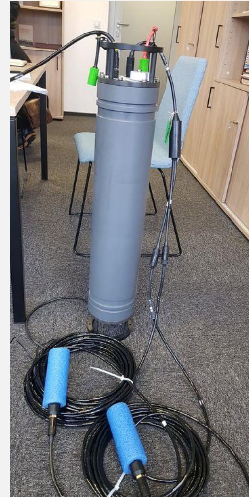
Hydrographic buoy for continuous underwater noise measurements with two hydrophones.
