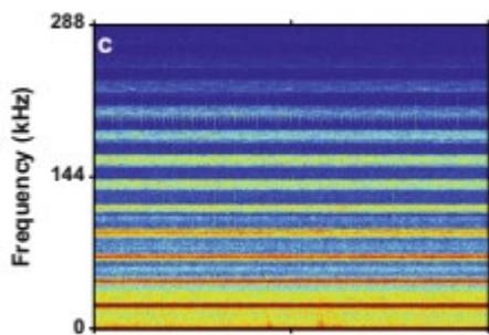
Fig. 2. Spectrogram of ultrasonic antifouling signals recorded from cruise ship *Oceania Regatta* (taken from Trickey et al., 2022)
