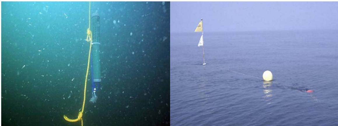
Fig. 1 : A POD moored under water. Fig. 3 Surface markers of a TPOD mooring in the Baltic Sea.
