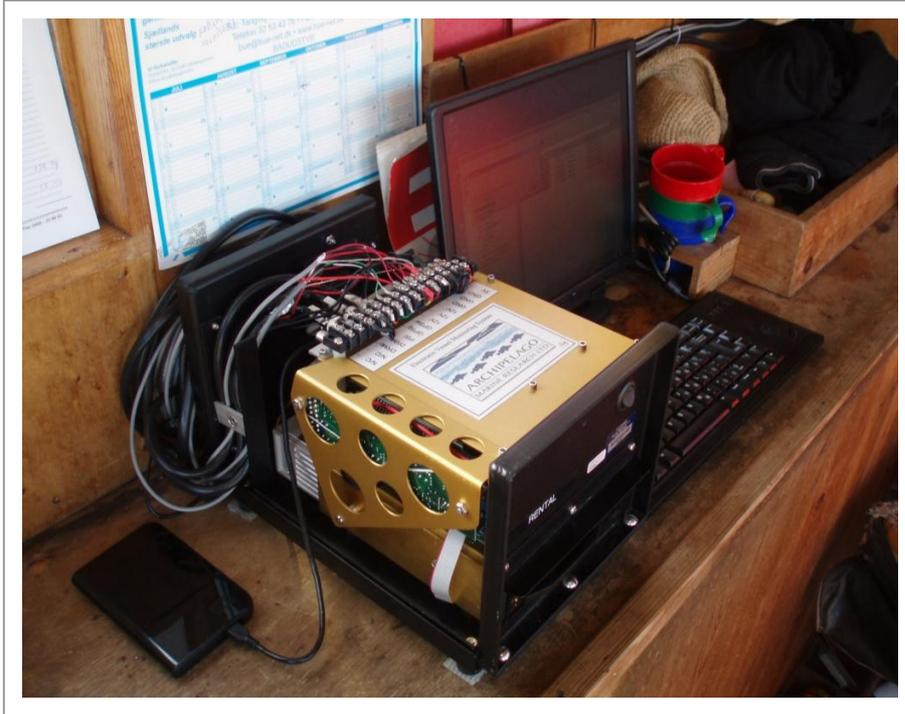
Plate 3. The EM box, with the cover removed and a portable external hard drive attached for downloading of data.
