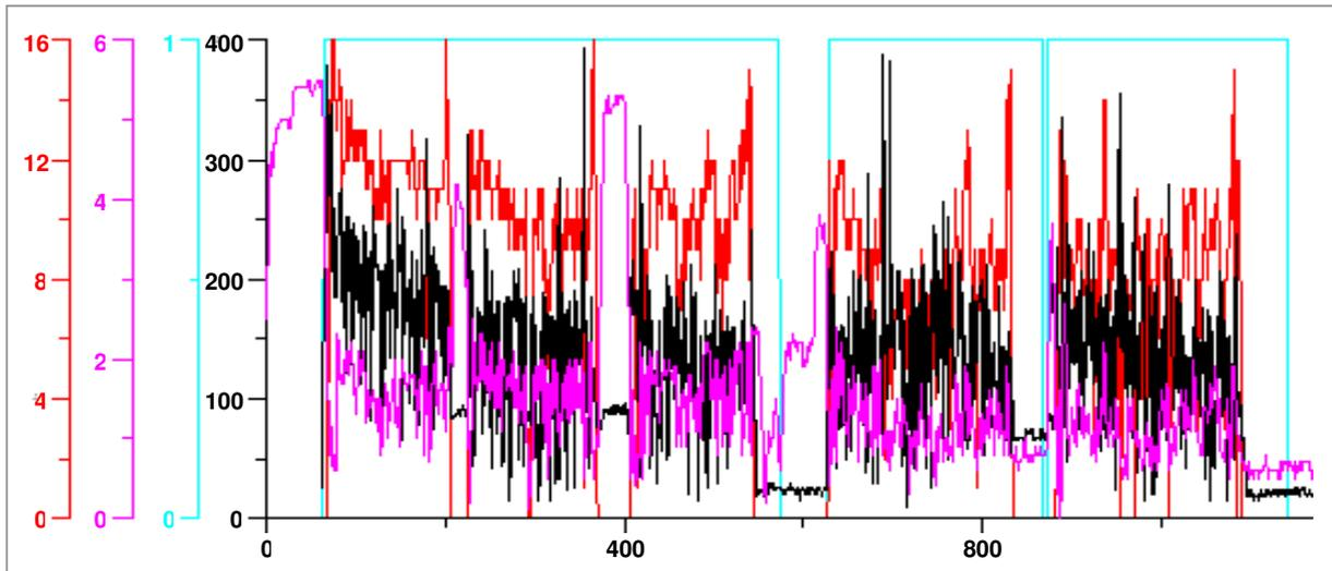
Fig 2. Fishing activities in graph form, showing five net haulings in one trip. On the y-axis, red represents the hailer drum rotations per 10 seconds, pink shows the vessel's speed in knots, light blue indicates when video data is recorded (=1) and black gives the hydraulic pressure in the hauler system (bar). The x-axis is time in 10 second units. In this sample, recording was programmed to start when the hydraulic pressure reached a certain threshold value.
