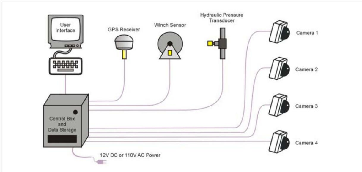
Fig 1. Schematic diagram of the EM system and its components.
