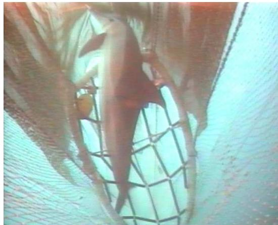
**Figure 50: Grid configurations tested in the flume tank of Boulogne, France by IFREMER - rigid version**
