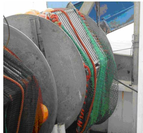
**Figure 2: Grid used in Swedish Nephrops fishery – on the netdrum**
