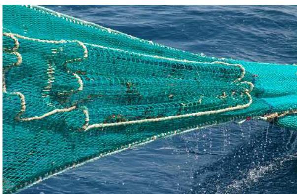
**Figure 6: SMP (100 mm mesh size) used in the Bay of Biscay**
