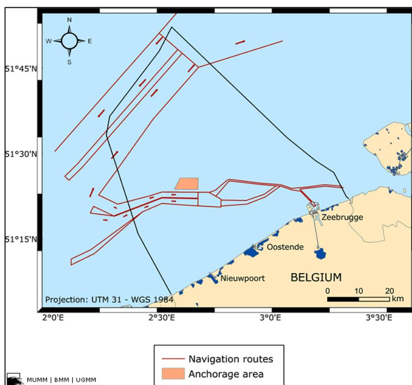
**Figure 1:** Shipping lanes in waters under Belgian jurisdiction. Large ships are bound by these shipping lanes; smaller ships with a more limited draught can navigate outside these lanes.
