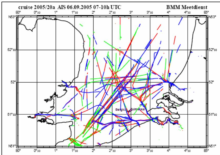
**Figure 2:** AIS data collected in 3 hours time by the BELGICA (ship's position indicated on the map); the green, red and blue lines represent respectively the tracks of ships equipped with AIS during the first, second and third hour of recording (from Backers, 2005).
