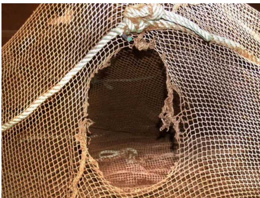
Figure 9.2. Typical predator hole in a net (photo credit: Knox Nets; taken from Northridge et al. , 2013).
