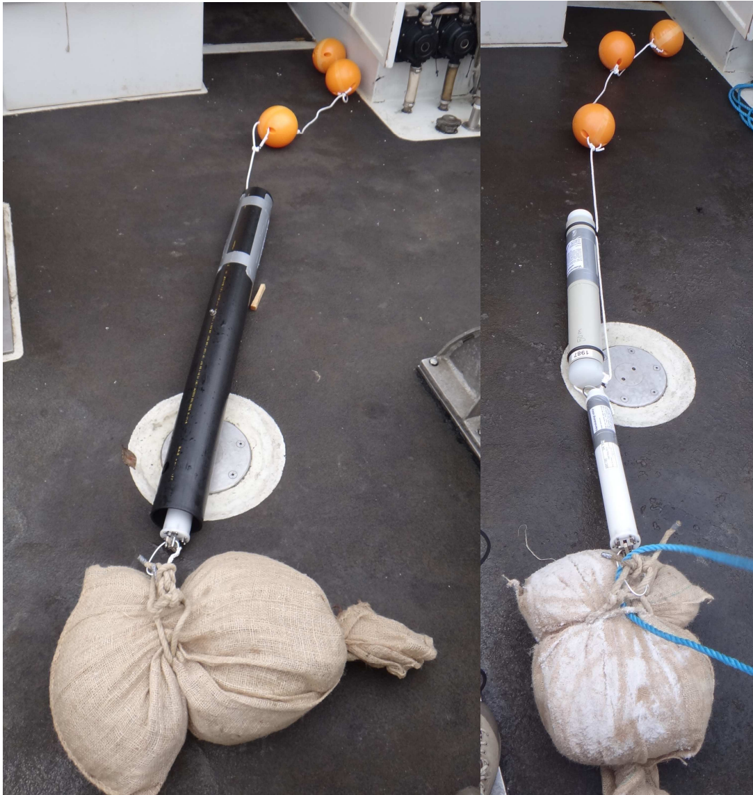
Figur 2.3.1 Acoustic equipment with and without protective tube with hydrophone at the top and acoustic release mechanism between tube and sand bag. Orange buoys keep the equipment vertical in the water column.
