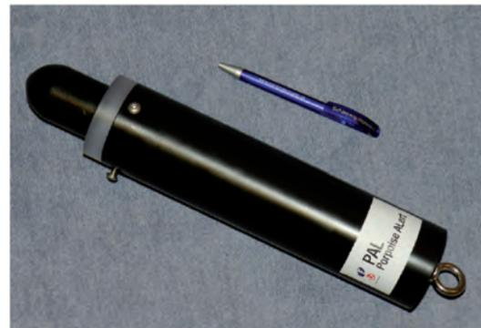
Figure 3 : Porpoise clicktrain generator PAL v1
