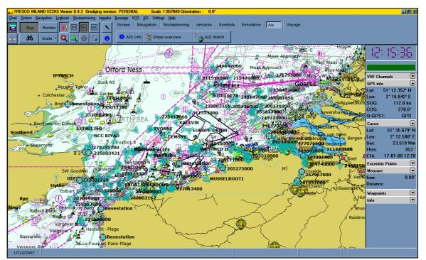
**Figure 3:** Ad hoc AIS image of the presence of ships in the southern North Sea and eastern Channel, as recorded from the aircraft OO-MMM on 17 January 2008, 12:15h UTC. The green/blue triangles indicate ships transmitting an AIS signal (the signals include their heading); for some ships the MMSI code is given, for others the name of the ship. The position of the aircraft is approximately 12 NM off the (shore) border between France and Belgium.
