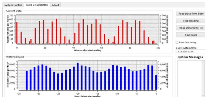
Fig. 3: Data visualisation on the receiver-PC. Red bars: minute sums of received clicks. blue bars: hourly click sums.
