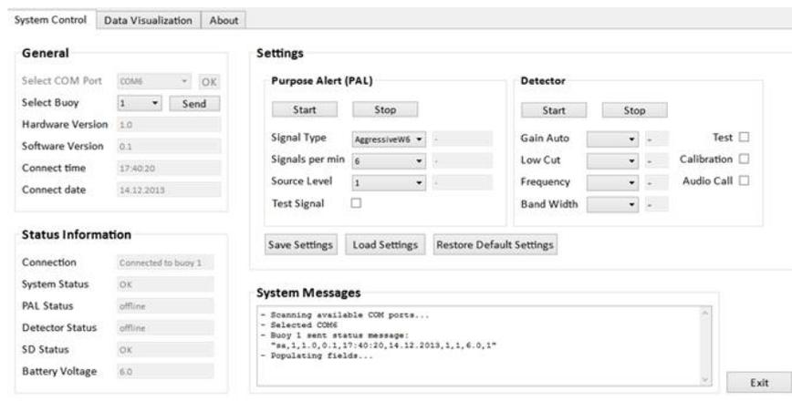
Fig. 2: Graphical user interface of PPD-receiver
