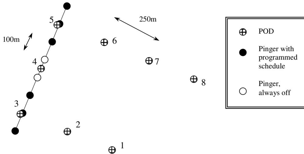
Figure 2. Three PODs (3-5) were placed on the simulated net and five single PODs (inshore southern row 1-2 and offshore northern row 6-8) were deployed at distances of 250, 500 and 750m and perpendicular to simulated net. The pingers were positioned 4m above the bottom and the PODs 2m.
