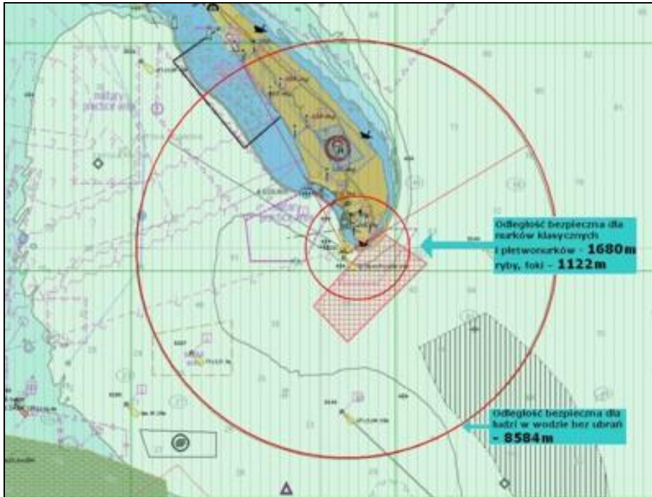
Fig. 3 The detonation location and the marked safety zone
