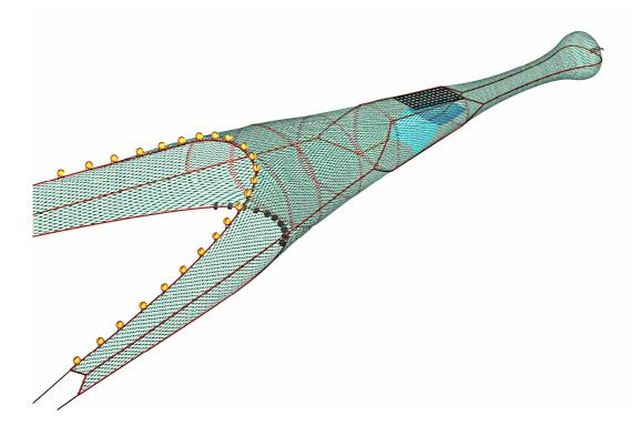
Figure 17: Diagram of experimental net with square mesh panel (black) and an inclined guiding panel (blue) underneath. A gap between the leading edge of the inclined panel and the belly netting allows prawns to pass under the guiding panel into the codend.
