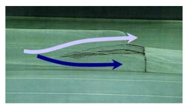
Figure 19: Inclined Separator Panel – model showing working principle. Light blue arrow is non-target species, dark blue is target species
