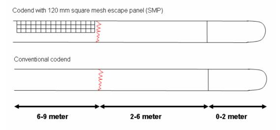
Figure 15: SMP and conventional codend used in Denmark
