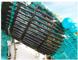
Figure 6: SMP (100 mm mesh size) used in the Bay of Biscay
