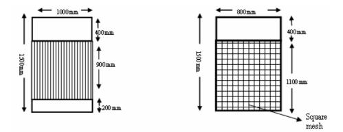
Figure 10: Grids (GCRUST2 and GCRUST3) tested in Portuguese Nephrops fishery - alternative designs
