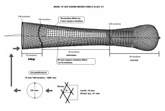
Figure 18: Model of SMP used in the Bay of Biscay
