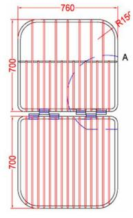
Figure 3: Grid used in Danish Nephrops fishery – model
