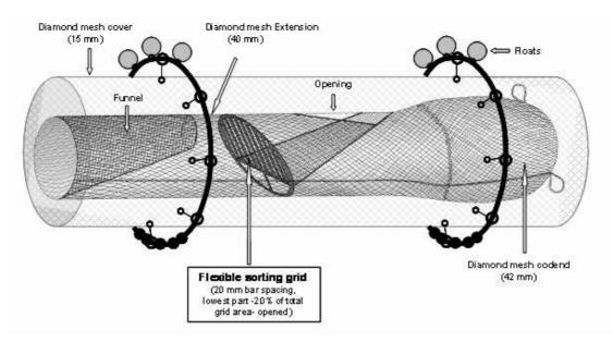
Figure 14: Sorting grid with guiding funnel used in the Catalan Sea
