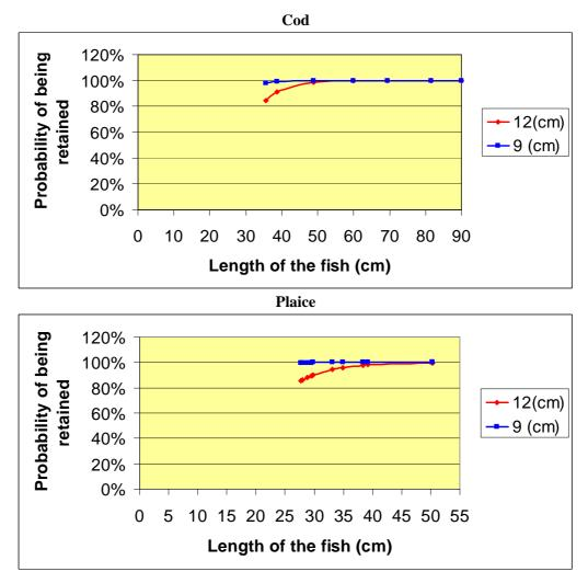
Figure 38: Selectivity curves for the Kattegat/Skagerrak trial (Source: the Danish NECESSITY trial team)
