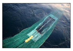
Figure 48: Escape holes designed by AZTI – sea trials
