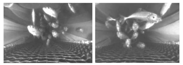
Figure 8: Underwater footage - French trials - horse mackerel swimming along with the gear in a collecting bag above the SMP
