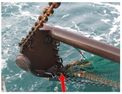
Figure 21: Lowered headline in Nephrops Beam Trawl
