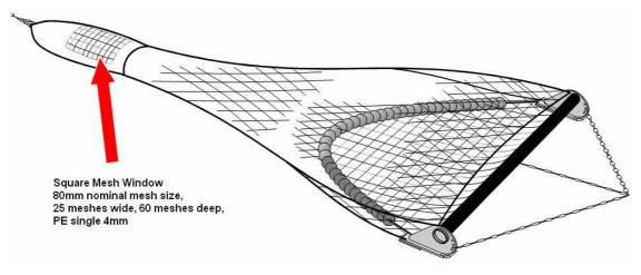
Figure 22: Square Mesh Window in Nephrops Beam Trawl
