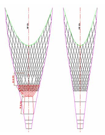
Figure 43: Tunnel barrier designed by IMARES and MARITIEM, tested on FRV "Walther Herwig -III" in 2006.
