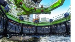
HSD-Net (Hydro Sound Damper) (reduces low frequencies)
