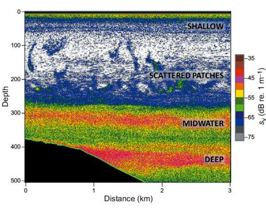
Three sound-scattering layers revealing patches of high prey biomass: 'shallow' – 30-90m depth, 'midwater' – 200-300 m depth, migrating vertically in 24-hr cycles, 'deep' – 350-450 m depth, no diurnal migration
